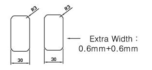
If your velcro tape is of 55mm width, we prepare knife size of 56.2mm including extra width(0.6mm+0.6mm, as shown in above image.) to cover tolerance of velcro tape. (in case of R=5mm) So, if your velcro tape has more tolerance than above, R=3mm is recommended.
